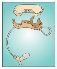
The two portions open to allow easy replacement of the 312 battery. The two portions also come apart to enable replacement of the Earpiece.
