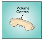
The Main Body is the portion of the hearing aid that houses most of the electronics. This piece connects to the Earpiece and includes the:
