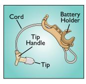
The Earpiece is the portion of the hearing aid that includes the battery holder, the cord, and the tip. This piece connects to the Main Body and includes the:
