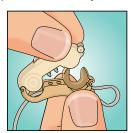
Remove the visible tab on the 312 battery and gently place the battery into the holder in the lower portion of the hearing aid. You will know that the hearing aid is facing the right way when the open bowl of the battery holder is facing you. Insert the battery with the plus sign "+" facing you. Gently close the two portions of the hearing aid. The hearing aid will not close if the battery is inserted the wrong way.
